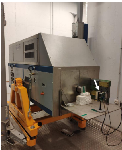
Fig. 4.. The sensor in front of Lillyput 3 accelerator output during the final radiation hardness test. The white arrow in the picture points to the sensor.
